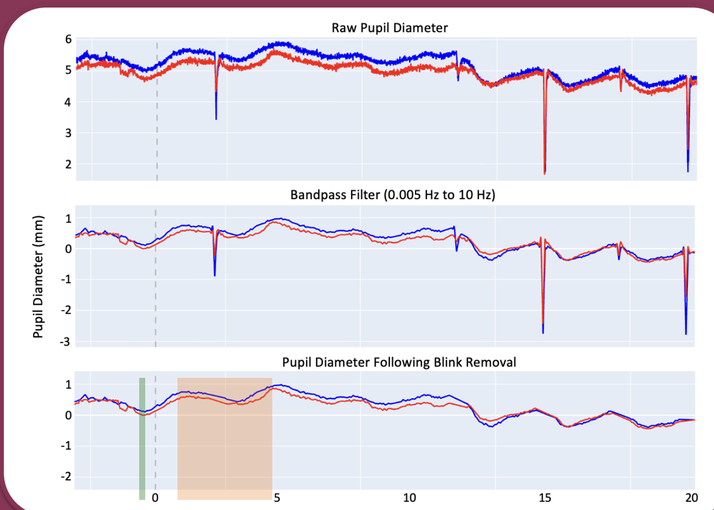
Fig 3. Traces of pupil diameter for a single trial. Top: Raw data; Middle: After bandpass filtering; Bottom: After blink detection and correction (linear interpolation). Orange box indicates 1-5s analysis window. Green box indicates 100ms baseline window.
